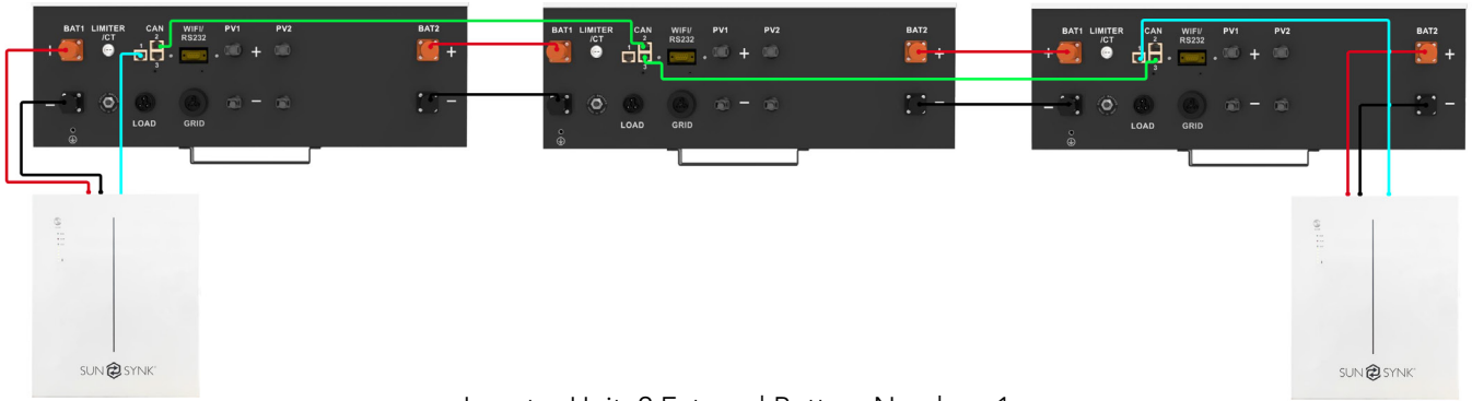
Inverter Unit: 2 External Battery Number: 1 (Shows CT Coil Connection + Master&Slave)
