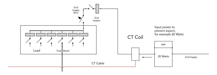
The CT coil is one of the most important parts of the LIFE3.6HYB02. This device reduces the power of the inverter to prevent feeding power to the grid. This is also known as zero export.
